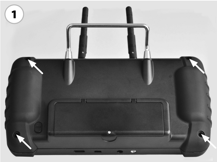
Open the cover of the transmitter by unscrewing the 4 screws as the picture shows.
